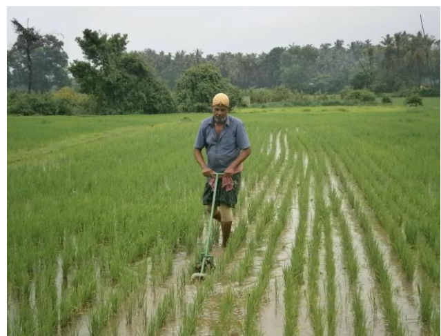
Figure 7. Cono-weeder used in rice in India
