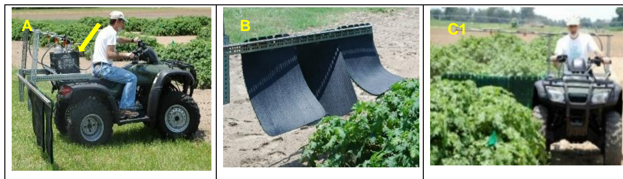
Figure 4. (A) The S-4 with a spray boom and abrasive mats fitted on one side of the ATV with the tufted, abrasive side of the mats facing forward and hung from a bar about 8 cm (3 inches) behind and below the spray boom. (B) The row of mats (shown back side facing the camera) were flexible as they passed over the TSA canopy. (C) Frontal (C1) and rear views (C2) of S-4 making passes over TSA plants.
