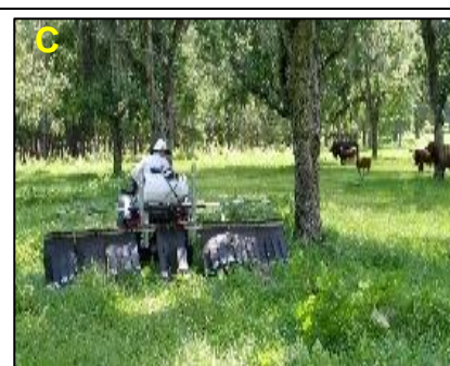
Figure 6. In M-1 modification of S-4, the mats were vertically cut into 11-cm (4.5-inch) strips, front ( A ) and back ( B ) views. The strips were attached and hung from a metal bar on an ATV as in S-4. ( C ) Application of SolviNix with M-1 in a TSA-infested mixed pasture-pecan grove.
