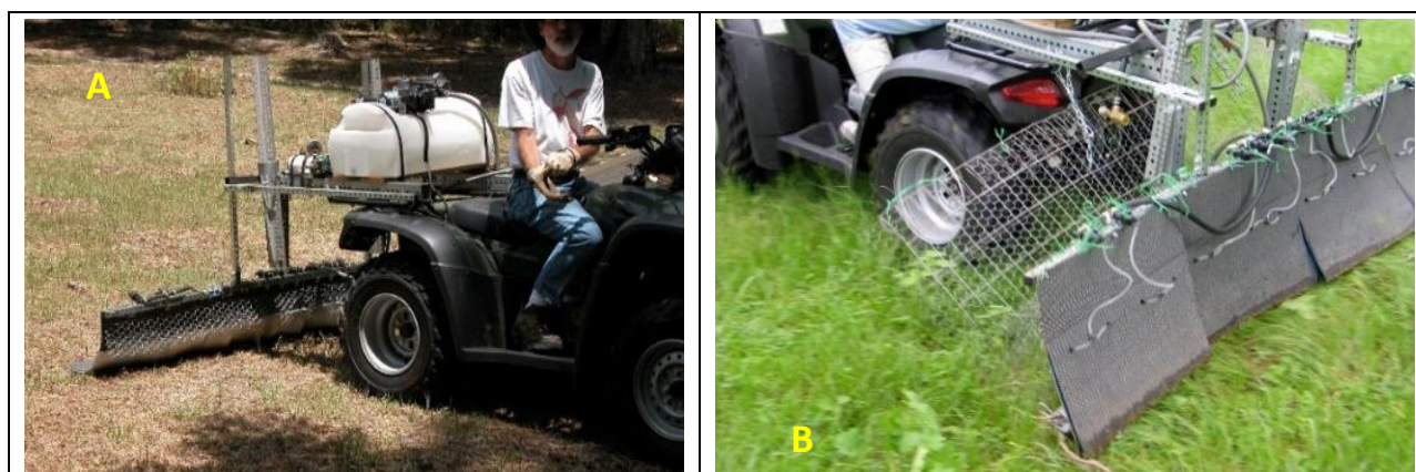
Figure 9. Modification M-1a to the Alley Cat herbicide wiper (S-5) with chicken-mesh fencing placed before the pad (A) and M-3a with galvanized reinforcement mesh and chicken-mesh before the pad (B), both modifications shown fully assembled and ready to be used.
