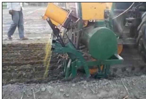
Figure 1. Lucky seed drill machine seeding the rice seeds and spraying pre-emergence herbicides in one pass. The optimum depth of seeding and uniform herbicide application is critical for establishing DSR with adequate control of the first flush of weeds
