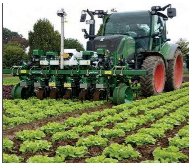
Figure 6 Robocrop Inter-row Cultivator (source: https://garford.com/products/robocrop-inrow-weeder/ )
