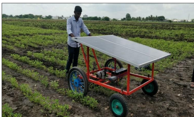
Figure 9 Solar-powered Weeder promoted in India to replace traditional tillage methods and fuel-driven equipment (Source: Kachhot, et al. 2020)
