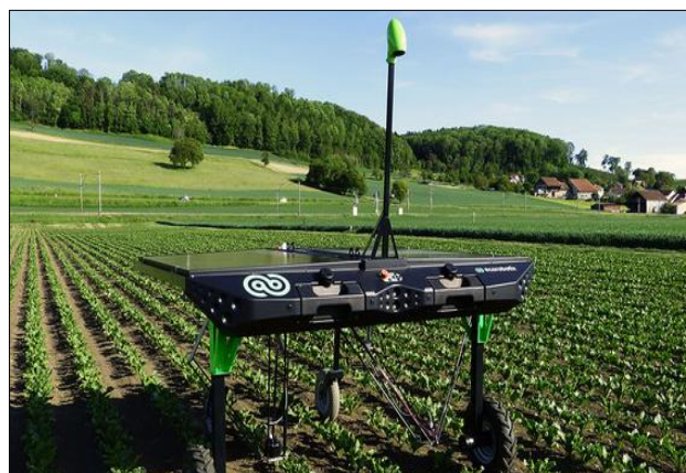
Figure 8 Solar-powered Robot used for herbicide spraying in row crops (Source: EcoRobotix (2022))
