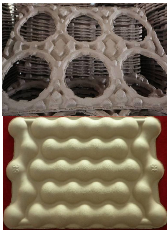
Figure 5. Wheel hub packing container (top) and back of fruit tray (bottom) made of mixed pulps containing smooth cordgrass fibres
