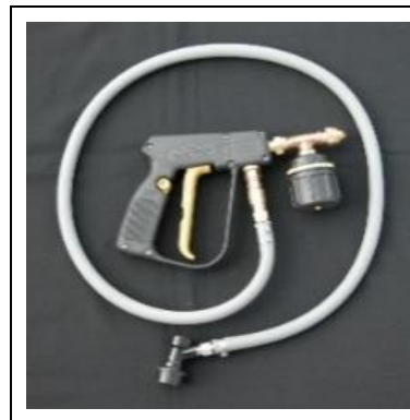
Figure 1. The S-1 sprayer gun for spot-spraying with a pre-set 2-mL volume of SolviNix per discharge at 0.55 MPa (80 psi).
