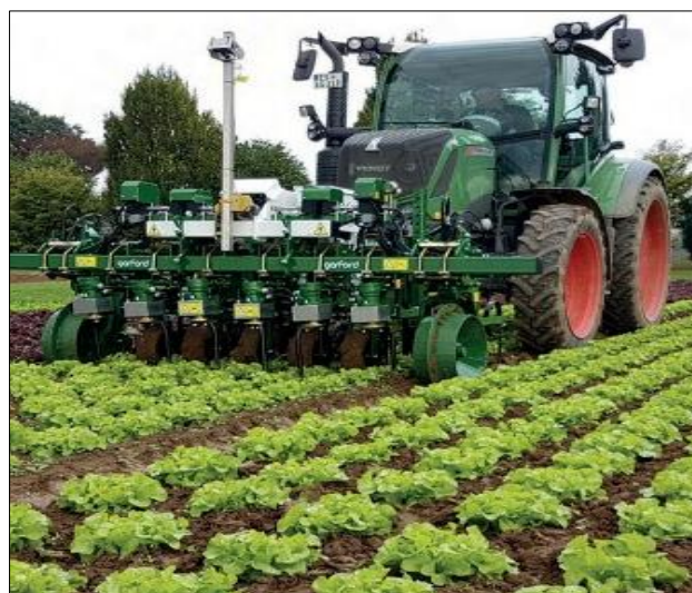
Figure 6 Robocrop Inter-row Cultivator (source: https://garford.com/products/robocrop-inrow-weeder/ )
