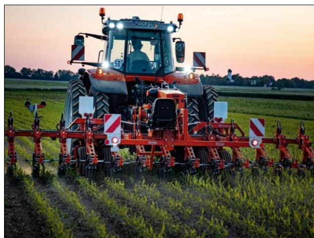
Figure 7 Steketee-IC 'Intelligent' Weeder for row crops (Source: https://www.steketee.com/about-us/ )
