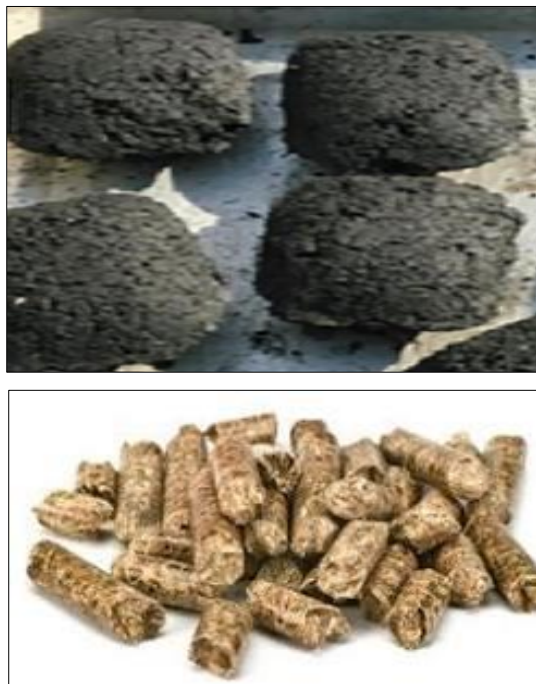
Figure 3 (A) An image of Bio-briquettes made up of WH charcoal and molasses (from Carnaje et al. (2018); (B) Bio-briquettes made with WH: EFB (from Rezania et al. (2016)
