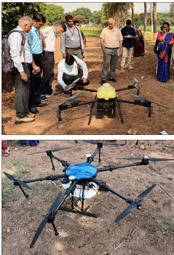
Figure 3 Drones being tested for herbicide spraying. Note the spray tank underneath and the nozzles attached to the wings
