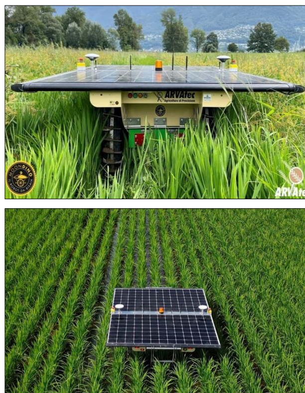
Figure 6 MoonDino Robotic weeder can be used for mechanical weeding immediately after sowing on dry and submerged land, with GPS-guided precision
