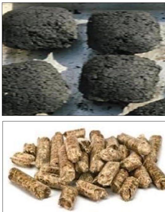
Figure 3 (A) An image of Bio-briquettes made up of WH charcoal and molasses (from Carnaje et al. (2018)); (B) Bio-briquettes made with WH: EFB (from Rezanja et al. (2016))
