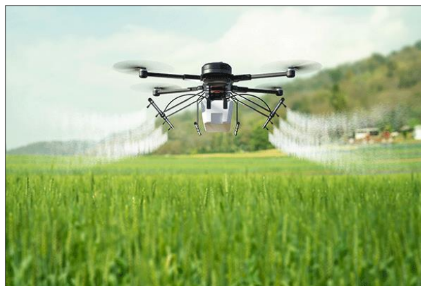
Figure 5 Unfavourable spray drift that can occur from a drone application with long booms (from Ozkan, 2024)
