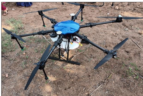
Figure 3 Drones being tested for herbicide spraying. Note the spray tank underneath and the nozzles attached to the wings
