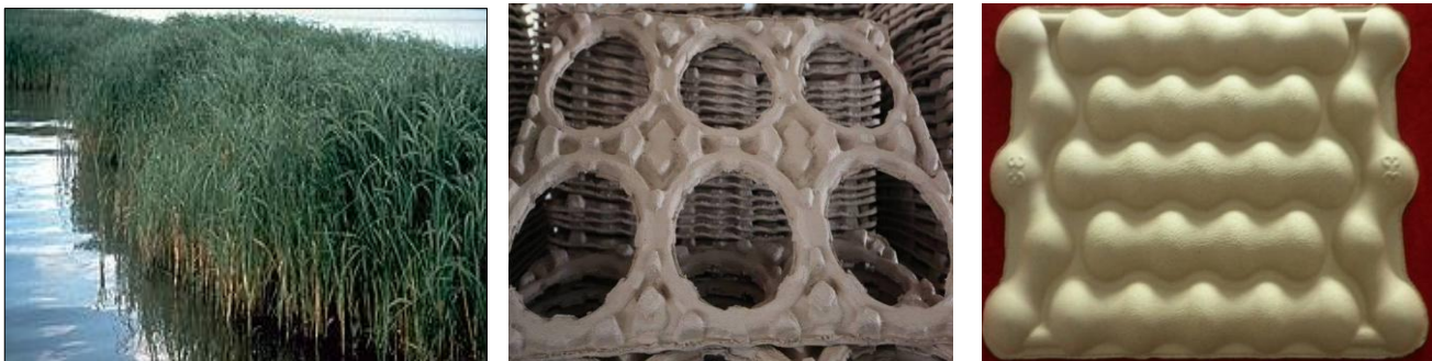
Figure 3. (a) Cordgrass infestations in China, (b) Wheel hub packing container (top) and back of fruit tray (bottom) made of mixed pulps containing smooth cordgrass fibres
