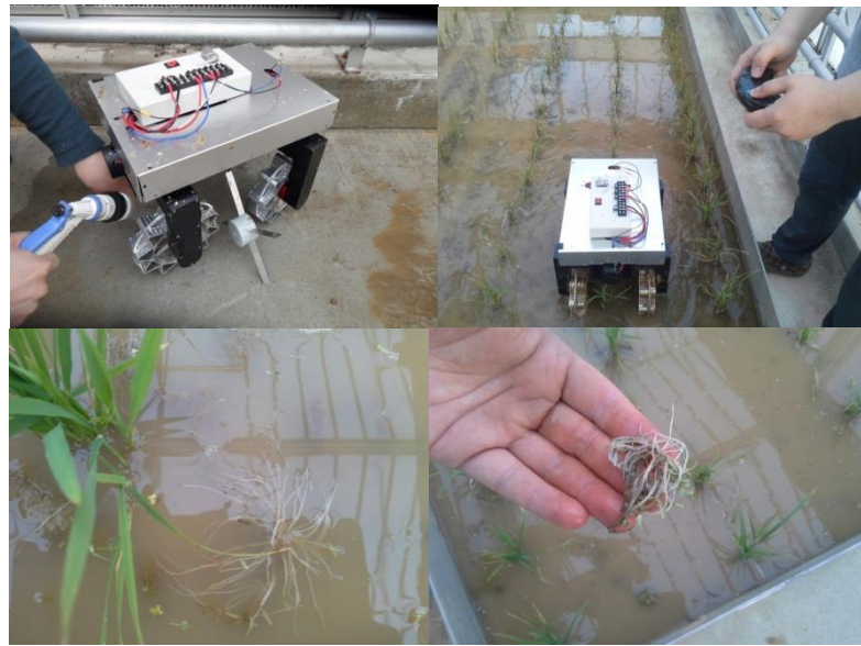
Fig. 7. A weed uprooted after operation by Robotic Weeding System
